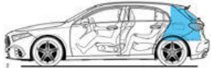
Open luggage compartment behind rear seat, loaded to roof, volume 435 litres (V 214-2)
